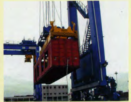
Figure 4: The sway control unit developed by Ruppel allows container cranes to work faster, so that the unit very soon pays for itself.
