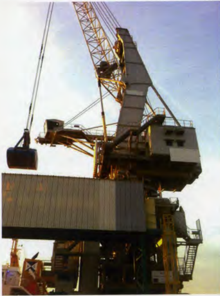
Figure 2: This automated crane used in bulk goods transfer required high levels of positioning accuracy for its derricking boom and grab.
